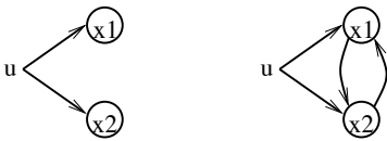
Fig. 3. Two possible networks corresponding to minimal realisations of the transfer function: decoupled (left) and coupled (right) internal structure.
